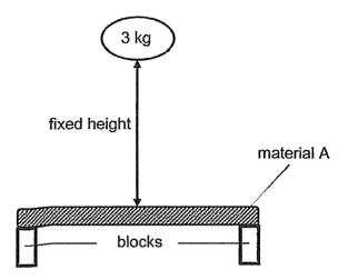
Gopal recorded the number of times the 3-kg weight was dropped before the material broke in the table below. He then repeated the experiment using materials B, C and D.
