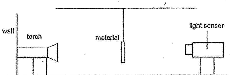
He placed each material between the torch and the light sensor and recorded the amount of light detected by the sensor. The table below shows his results.
