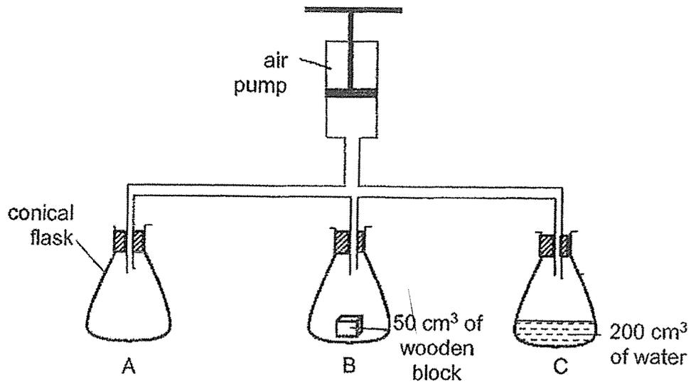
The handle of the air pump is pushed down three times, pushing in 100 cm<sup>3</sup> of air with each pumping action.
