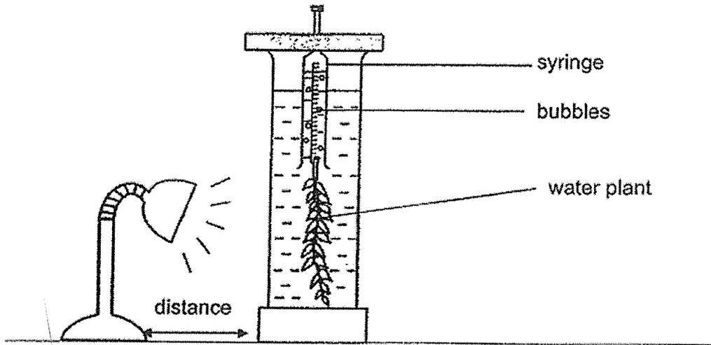
He measures the volume of gases collected in the syringe at various positions of the lamp and records the results as shown below.
