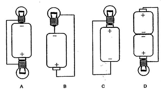
Which circuit(s) will <u>not</u> allow electric current to flow through to light up the bulb(s)?
