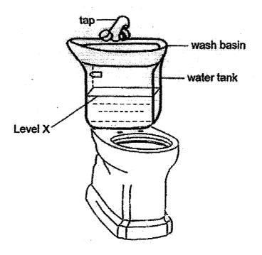
After flushing, water refills the tank and the tank will stop filling when the water reaches level X.
